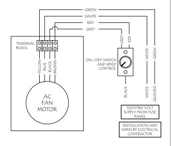
VARIABLE SPEED CONTROL DIAGRAM NOT TO SCALE
