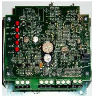
Figure 22 - Flame Safety Controller
