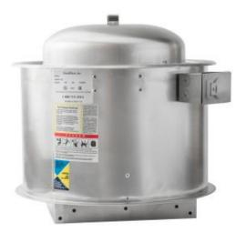
NAKS DECA series (UL762) is ideally suited for removal of grease laden exhaust found in restaurants and commercial kitchen applications. All DECA models are designed to handle 300°F flare up per UL762 and maintain a minimum 500 FPM air flow in duct. Other applications include a wide range of commercial, industrial, and institutional facilities such as schools hospitals, and assembly areas. Add the wall adapter option and the uses of our DECA
