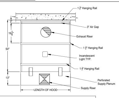
It is the responsibility of the architect/owner to ensure that the hood clearance from limited-combustible and combustible materials is in compliance with local code requirements
