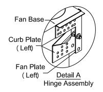
Step 1 - Line up the Fan Plate with the Fan Base as shown in picture 1.
