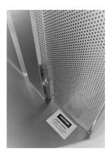
HoodMart's Short Cycle Makeup Air with IPS (Internal Perforated Supply) removes grease laden vapors from the air while replacing air without causing negative air pressure. This allows using a fresh air makeup air fan instead of a costly tempered air unit. IPS (Internal Perforated Supply) takes advantage of the Coanda Effect created inside the hood, further assisting with capture and containment
