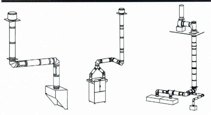
A MAJOR CAUSE OF VENT RELATED FIRES IS FAILURE TO MAINTAIN REQUIRED CLEARANCES (AIR SPACES) TO COMBUSTIBLE MATERIALS. IT IS OF THE UTMOST IMPORTANCE THAT NAKS SYSTEMS BE INSTALLED ONLY IN ACCORDANCE WITH THESE INSTRUCTIONS.
