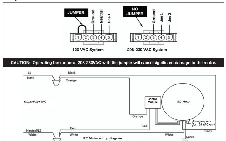
**NOTE:** EC motors have a soft start feature. When the power is turned on the control module gathers information from the motor then begins the start up process. After a few seconds the motor will start to turn and reach full set speed in 10-30 seconds.
