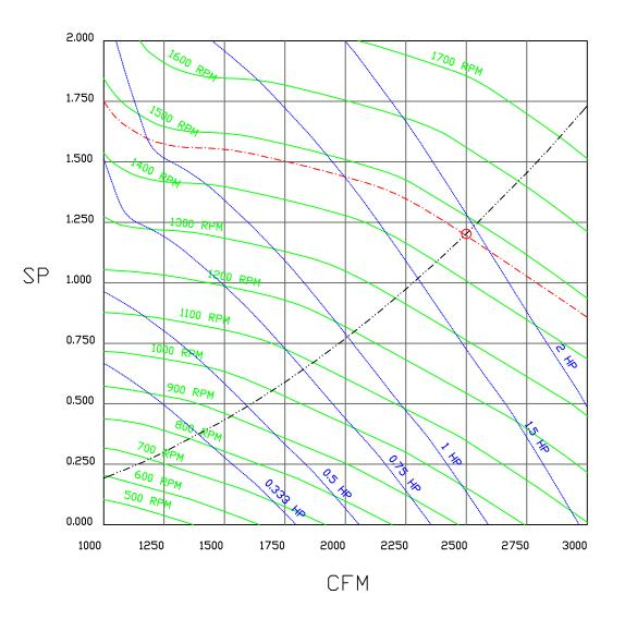
2500 CFM, 1.202 SP @ 1470 RPM and 1.872 BHP at 0 feet and 100 deg F \* Please note that these curves were adjusted for job specific temperature and altitude.
