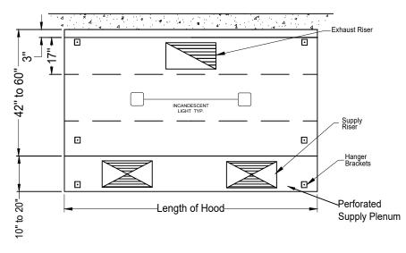
It is the responsibility of the architect/owner to ensure that the hood clearance from limited-combustible and combustible materials is in compliance with local code requirements
