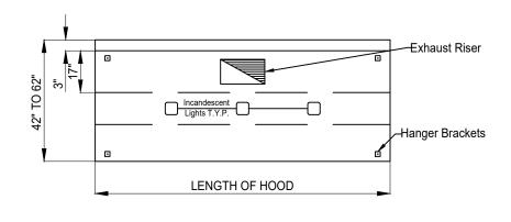
It is the responsibility of the architect/owner to ensure that the hood clearance from limited-combustible and combustible materials is in compliance with local code requirements
