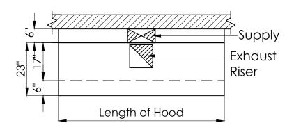
It is the responsibility of the architect/owner to ensure that the hood clearance from limited-combustible and combustible materials is in compliance with local code requirements
