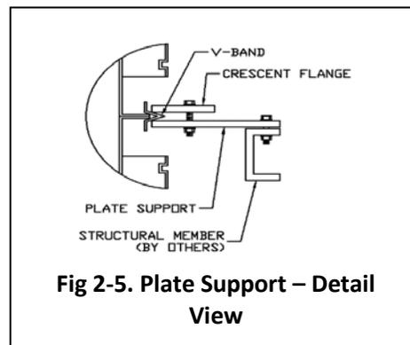
Fig 2-5. Plate Support - Detail View
