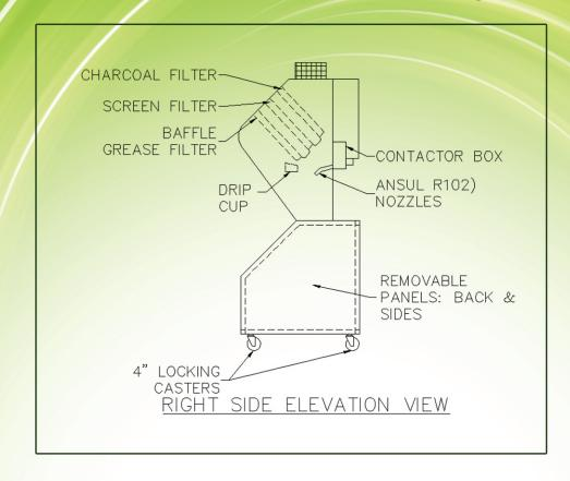
The Ventless Exhaust Hood System is approved for electric equipment and fryers with oil capacities of up to 85 pounds; not to exceed 470 square inches of cooking area.
