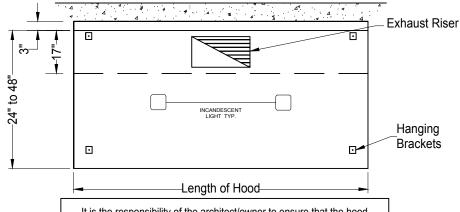
It is the responsibility of the architect/owner to ensure that the hood clearance from limited-combustible and combustible materials is in compliance with local code requirements
