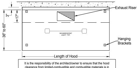
clearance from limited-combustible and combustible materials is in compliance with local code requirements
