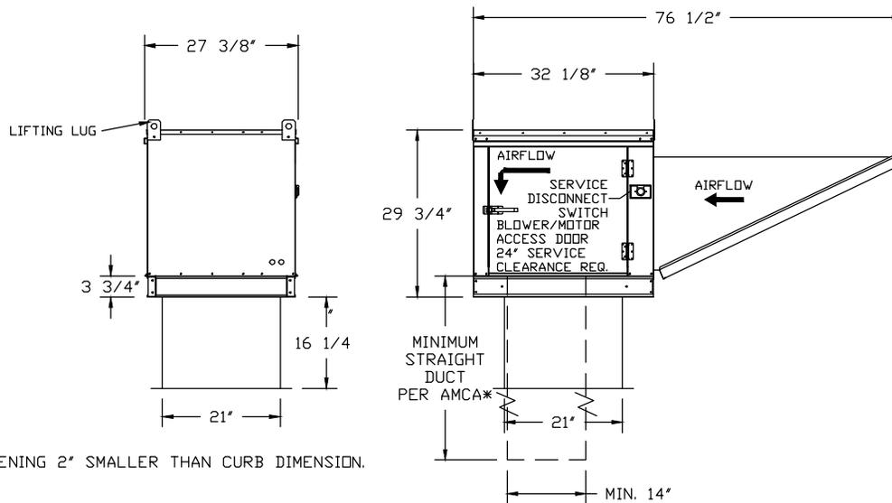
ROOF OPENING 2" SMALLER THAN CURB DIMENSION.
