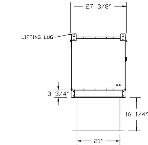
ROOF OPENING 2" SMALLER THAN CURB DIMENSION.
