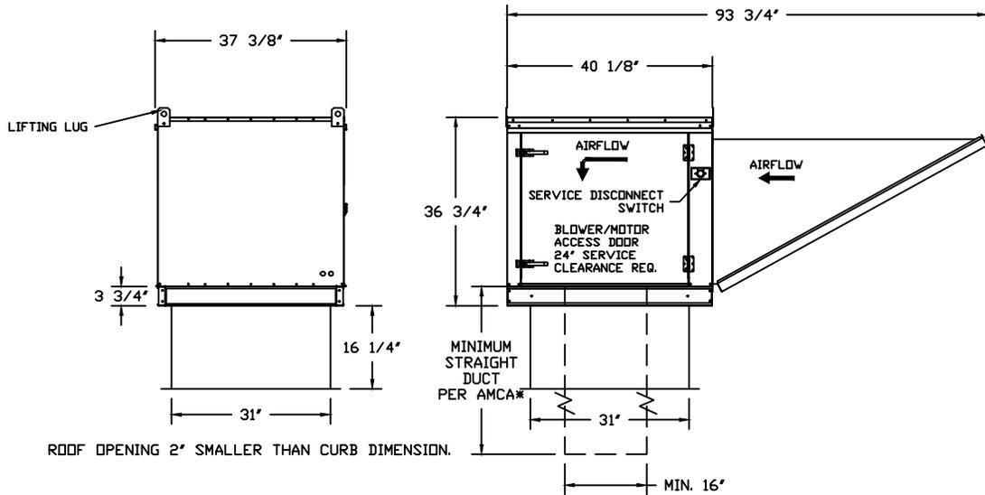
ROOF OPENING 2" SMALLER THAN CURB DIMENSION.
