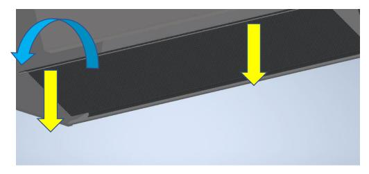
Rotate IPS down by pulling on trim strip where indicated (be cautious to avoid damage to hood and IPS).
