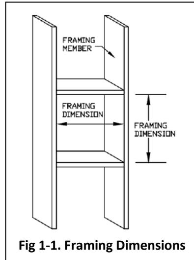
**Fig 1-1. Framing Dimensions**
