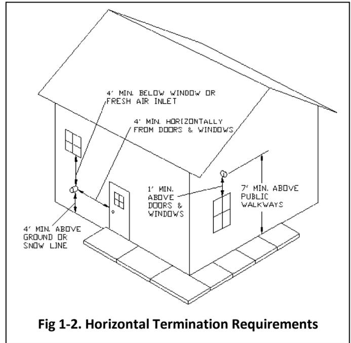
Fig 1-2. Horizontal Termination Requirements
