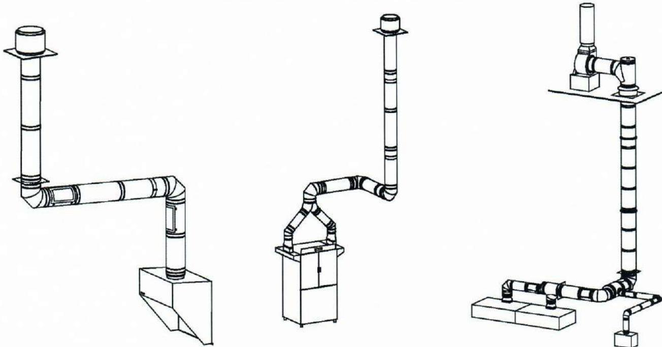
**A MAJOR CAUSE OF VENT RELATED FIRES IS FAILURE TO MAINTAIN REQUIRED CLEARANCES (AIR SPACES) TO COMBUSTIBLE MATERIALS. IT IS OF THE UTMOST IMPORTANCE THAT NAKS SYSTEMS BE INSTALLED ONLY IN ACCORDANCE WITH THESE INSTRUCTIONS.**
