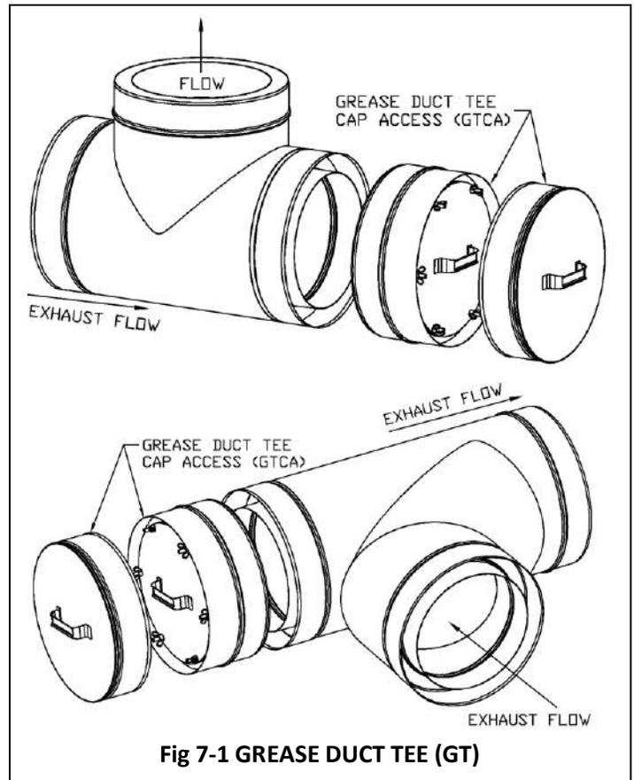
Fig 7-1 GREASE DUCT TEE (GT)
