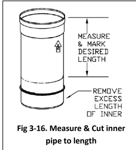
Fig 3-16. Measure & Cut inner pipe to length
