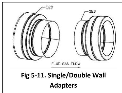
Fig 5-11. Single/Double Wall Adapters
