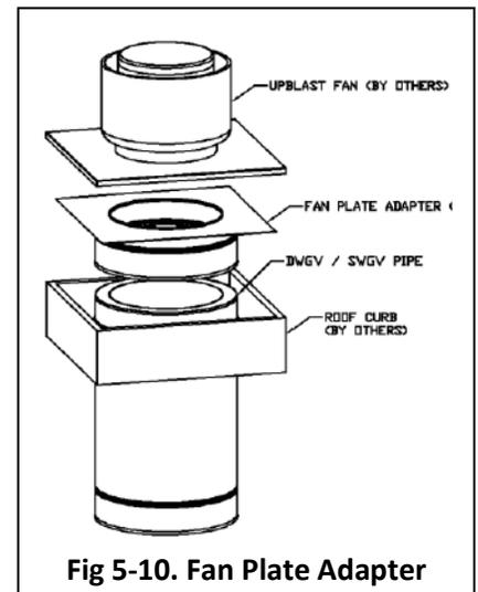
Fig 5-10. Fan Plate Adapter
