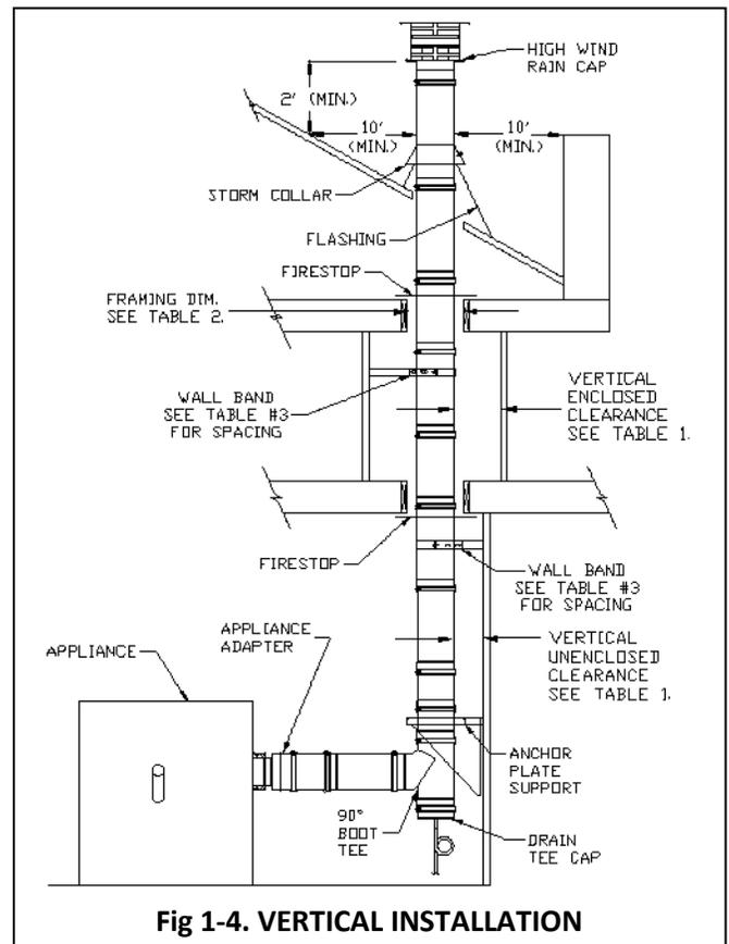
Fig 1-4. VERTICAL INSTALLATION
