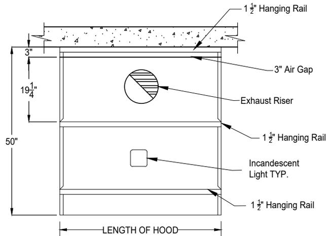
It is the responsibility of the architect/owner to ensure that the hood clearance from limited-combustible and combustible materials is in compliance with local code requirements
