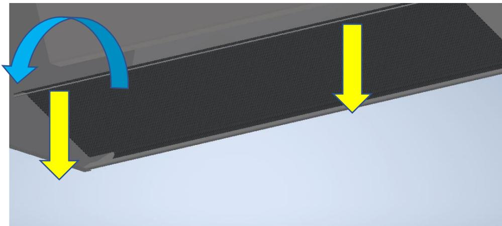
Rotate IPS down by pulling on trim strip where indicated (be cautious to avoid damage to hood and IPS).
