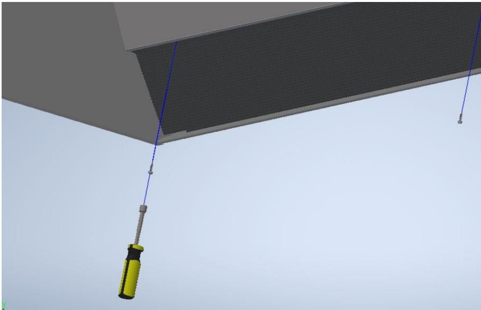
Use 5/16" nut driver to remove #8 hex head screws from IPS.
