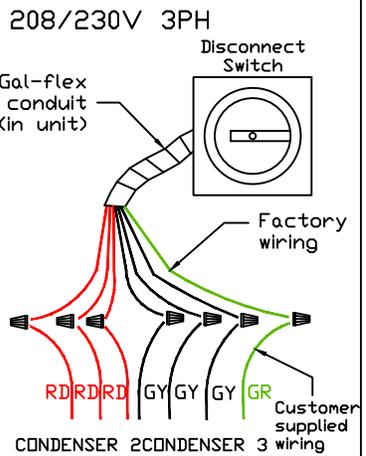
DO NOT CONNECT CONDENSER POWER DROPS TO KITCHEN CONTROL PACKAGE STARTERS OR VFDS
