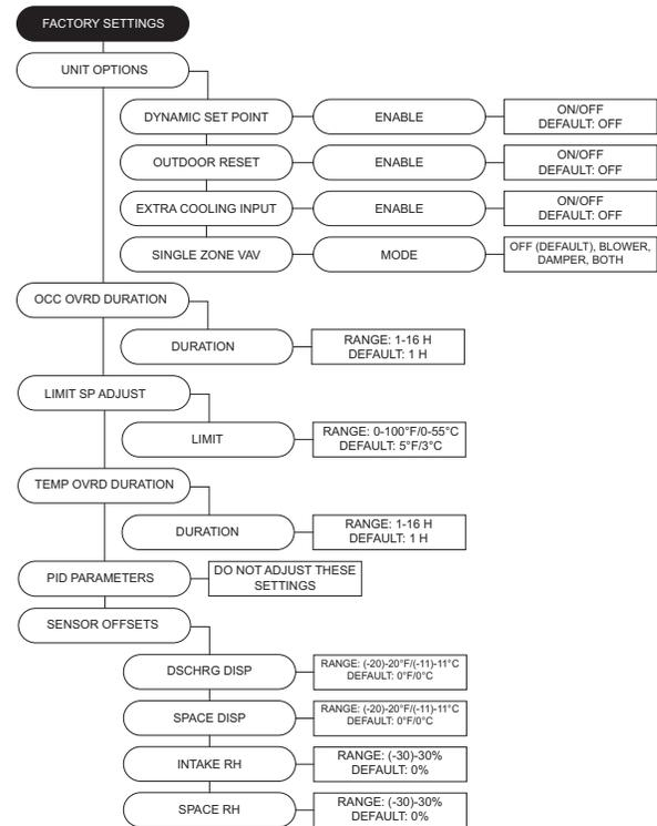
**NOTE: For every adjustment in Dynamic Set Point (SP) Differential, this would multiply the effect of the Dynamic Offset setting.**
