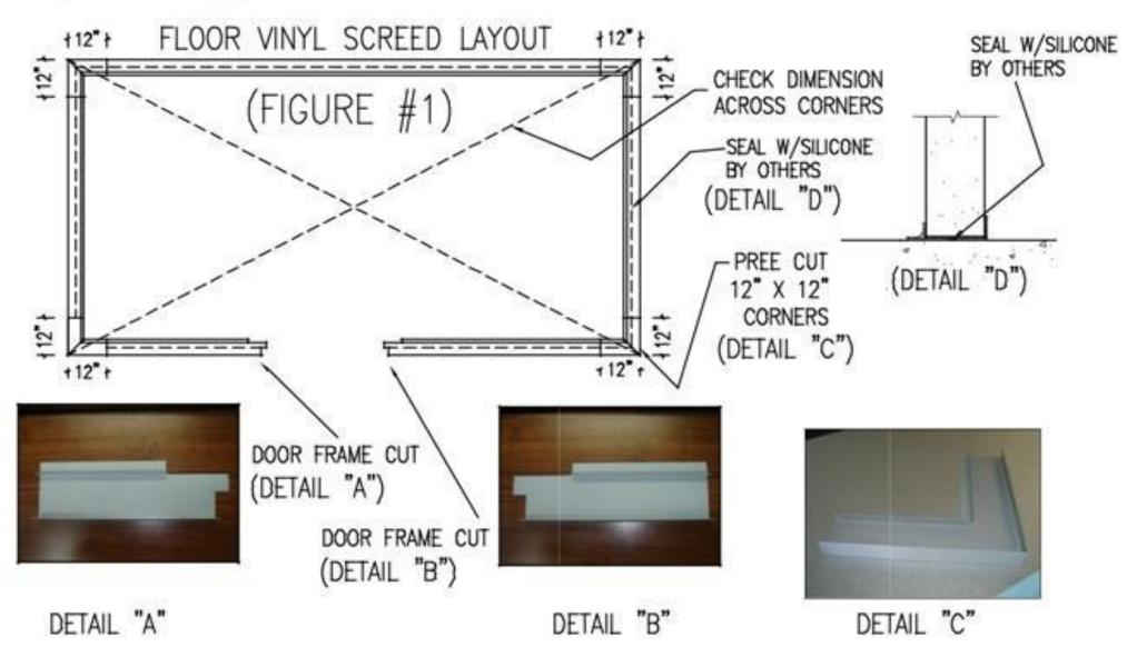
2-APPLY A BEAD OF SILICONE ALONG THE BOTTOM OF THE VINYL SCREED. THEN PLACE THE VINYL SCREED ALONG THE CHALK LINES.
